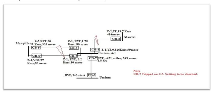
As per DR Analysis, Double phase to earth fault was in 132 kV Mawphlang - Umiam Stg I D/C Line and 132 kV Mawlai - Umiam Stage I Line at 10:23 Hrs of 24/4/23 and faults cleared from Umium stage-1 within 99 msec on Z-1 operation. At the same time, healthy 132 kV Umium Line tripped only from Umium stage-1 on I>3 (Ib:1.8 kA).
